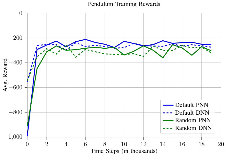
Fig. 3: The average episode reward obtained using the PNN network and DNN network on Pendulum. Rewards are shown in both Default training setting and Random training setting. We plot the average over 3 experiments of the average episode score evaluated every 1000 time steps.
